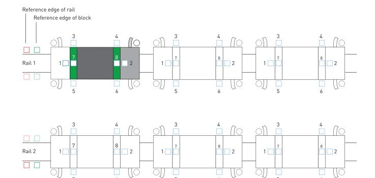
If the  $E_{1/2}$  dimensions are not indicated, the maximum possible number of mounting holes will be determined under consideration of  $E_{1/2}$  min and will be carried out symmetrically.
